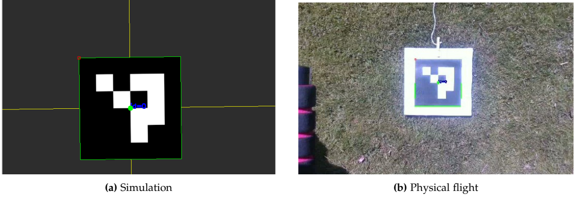
Figure 8.2: Successful detection of the 4 \times 4 ArUco ID 0 marker in simulation and in physical flight. Because the synthetic camera and the real camera publish to the same ROS 2 topic and are geometrically identical, the detector code is unchanged between the two environments.
